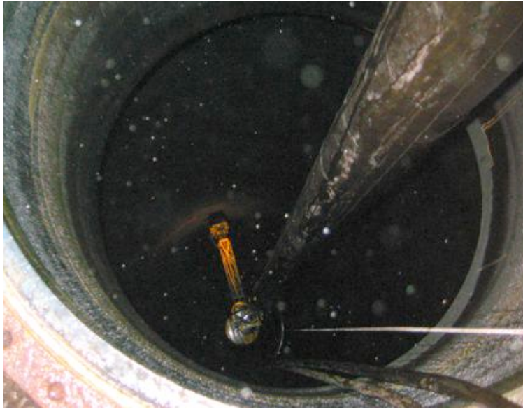
Crawler in action in the drum. Attached to drill stem, and scanning a circ weld.
