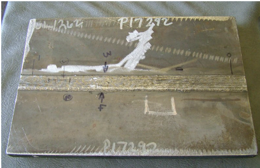
Figure 5: Test sample for ACFM experiments
